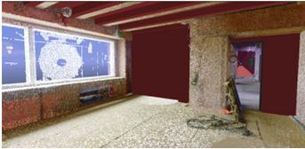
1) Example of digital twin with point clouds and simple BIM objects.
